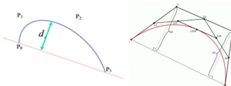
Figure 6 Maximum Transverse Deviation and Approximate Measure
