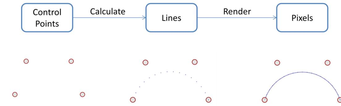
Figure 3 Flattening and rendering Bézier curve
