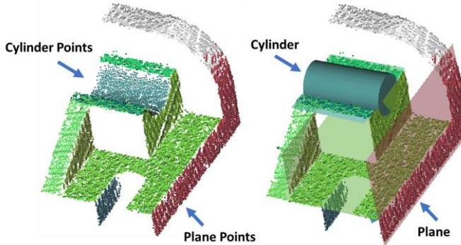
**Figure 4:** Detected shapes example. Left: inlier points for each shape are given different color. Right: some examples of the detected shapes.
