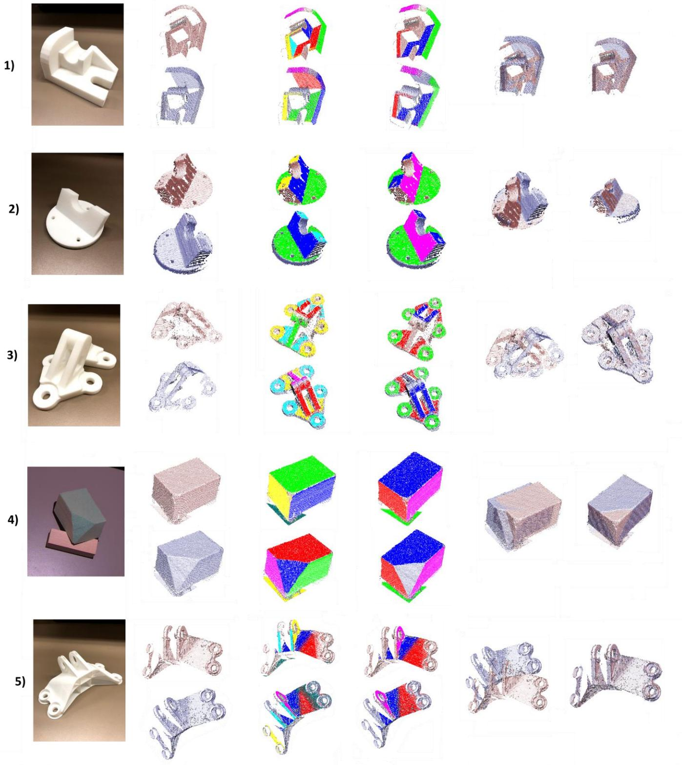
Figure 6: Five examples of aligning CAD point-clouds.
