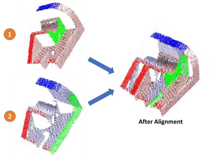
**Figure 5:** An example of a wrong random combination of basic shapes. After alignment the orthogonal distance between the basic shapes (the red, green and blue planes in this case) is almost zero, but the total distance (point to point) between the two point-clouds is large.
