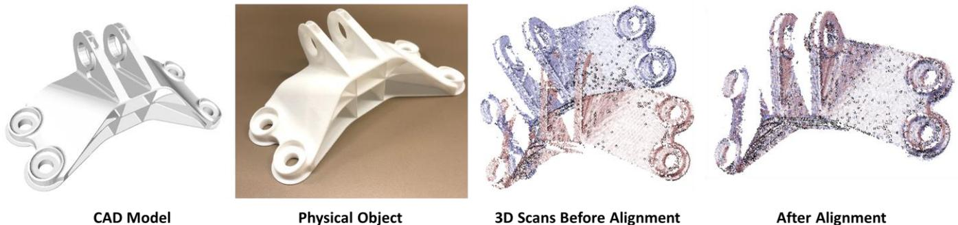
**Figure 1:** An example CAD object, 3D scanned from two different viewpoints, and aligned using our method
